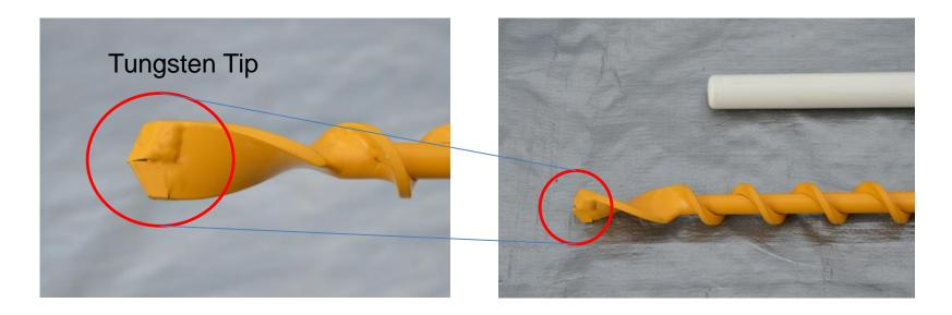
The auger is a little bit longer than the probe. The tapered soil opening created by the auger is therefore deeper compared to the length of the probe body. The resulting soil cavity below the bottom of the probe is designed to accept soil accumulating at the bottom of the cavity during the augering process. Otherwise soil accumulation could obstruct the insertion of the probe body to its full length.
