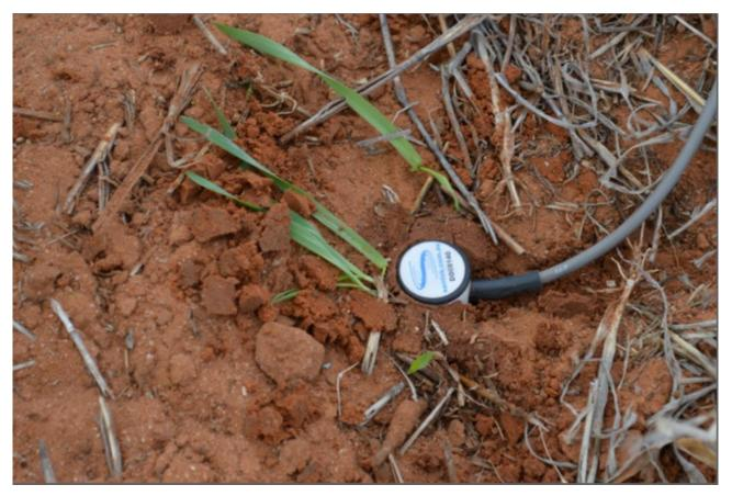
The almost-completely installed 30cm probe. The probe cable can be fitted with protective electrical cable conduit and buried adjacent to the probe. The greater length of cable can be left on the surface for convenient removal at times of farm machinery traffic.
