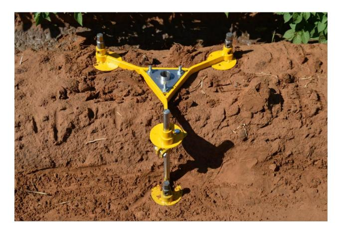
Two tripod feet are secured on top of the hill, while the tripod extension foot is secured at the bottom of the furrow.
