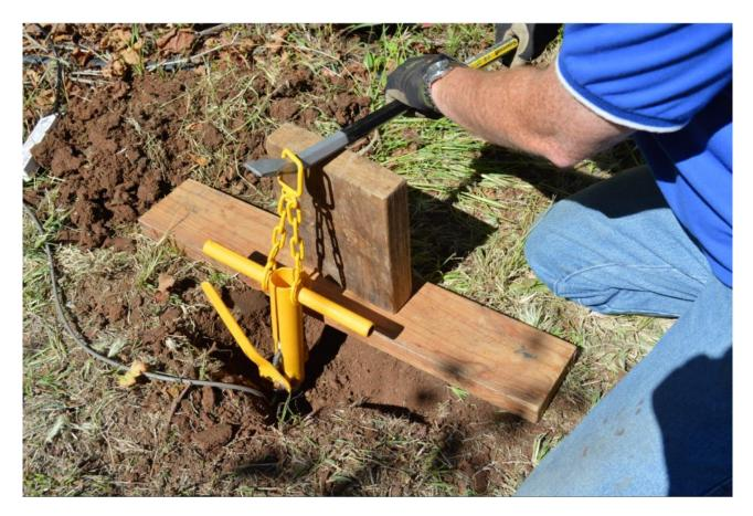
Locate the square ring on the crowbar and apply tension.
