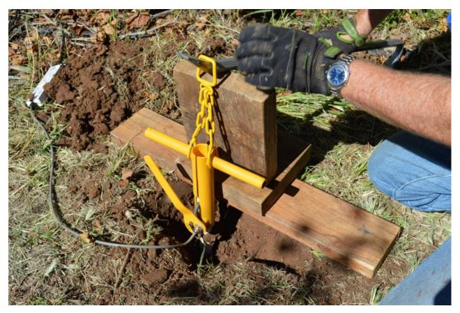
Apply downward force to the crowbar until the probe lifts a little bit and the tight bond between probe and soil is broken. Adding a little water to the probe and allowing it to infiltrate will aid removal.
