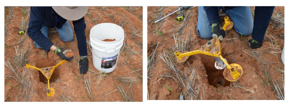
Before removing the tripod, remove any soil that may have landed in the hole around the Extension Tube. This will protect the augered probe hole during disassembly.
