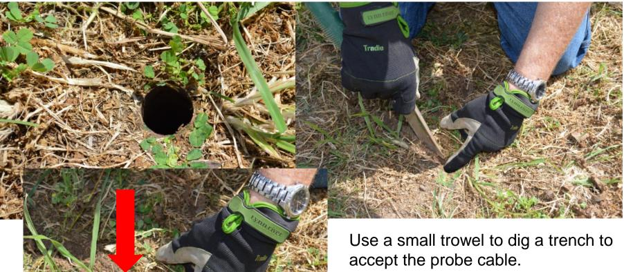
During excavation place your finger over the hole to prevent the soil falling into it.
