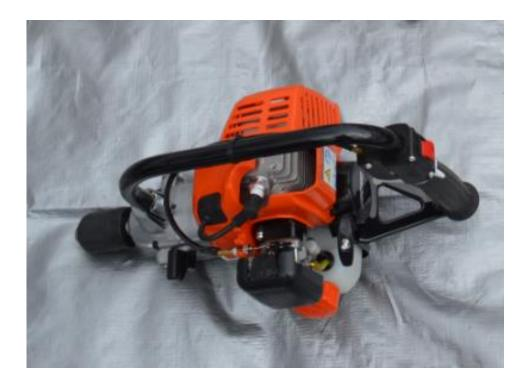
Alternatively, a motorized power head may be used to drive the tapered auger. The one shown is an ECHO EDR-2400 2-stroke engine drill by Yamabiko Corporation.
