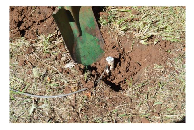
Excavate soil adjacent to the probe to a depth of 20 cm. Wipe any soil or water from the probe using a piece of cloth.
