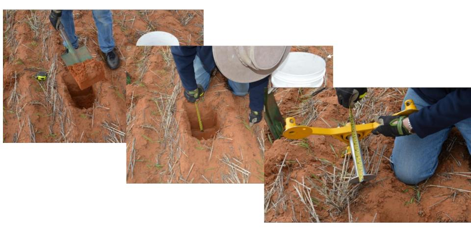
Excavate the soil to the correct depth. Ensure that the bottom of the hole is level.
