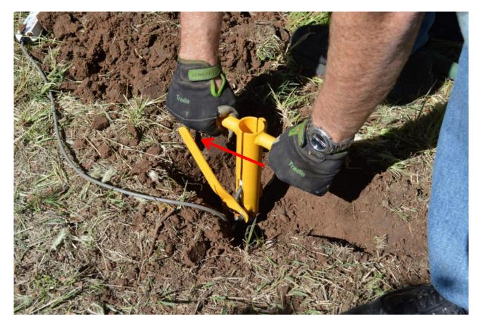
Move the lever of the tool from right to left as far as possible and then grab the tool handle and pull with a <u>gentle</u> twisting motion to remove the probe.
