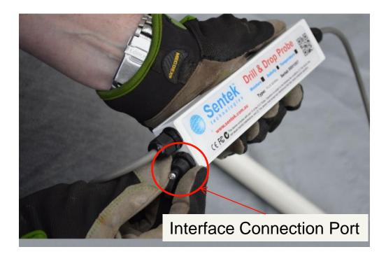
The interface box can be laid on the ground for convenient connection of a probe configuration cable, should the need arise. It may also be buried for protection from passing farm machinery or animal interference. Ensure that the probe connection port is tightly sealed with the cap provided. The probe installation is now complete and ready for connection to the logger.
