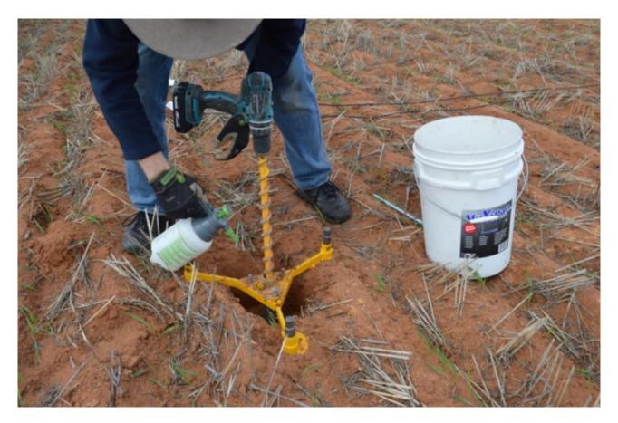
Use a water spray bottle to lubricate and pick up the drilled soil. Auger in short stages (30 – 50cm at a time), clearing the auger flights regularly. The excavated soil should be moist to maintain the integrity of the hole. Dry soil will collapse inward and lead to air gaps and failure of probe insertion.
