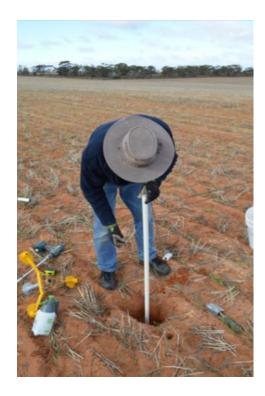
Spray water onto the surface of the probe and a little directly into the augered hole. Then immediately and smoothly insert the probe to maximum depth by hand.
