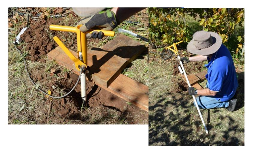
Gently remove the Drill & Drop Probe when it becomes free of the soil.
