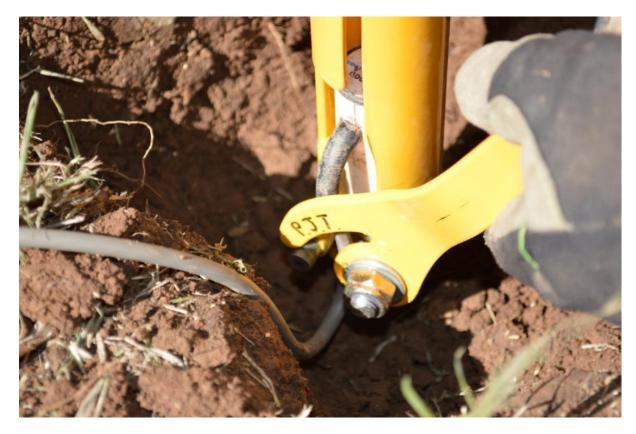
Fit the Extraction Tool around the probe so that it is at least 2 cm below the cable entry point.
