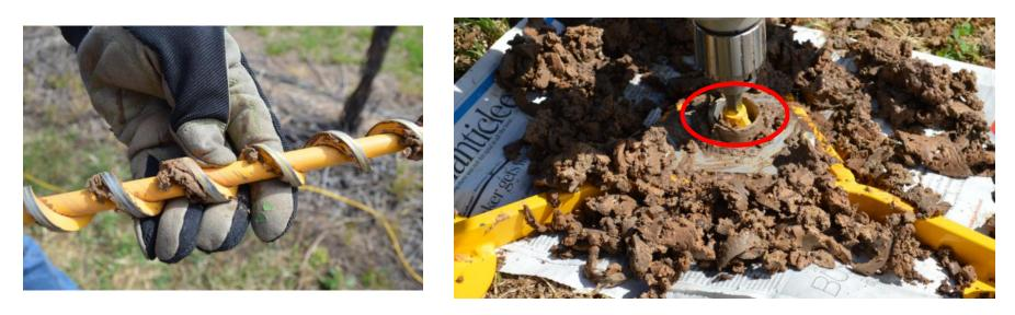
Now reintroduce the auger carefully with the drill switched off. Push auger until the top end of the flight is level with the hole of the tripod. If the auger will not go down to this level, give the auger a quick spin to take up the soil at the bottom of the hole, then stop the drill, remove it from the hole and clean it once again.
