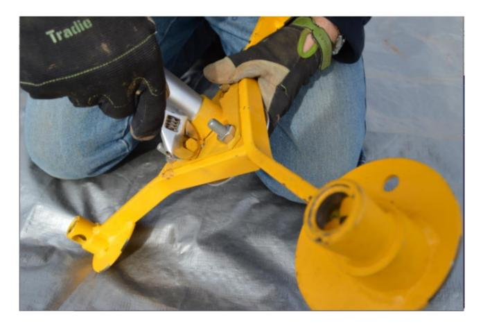
Loosen the Extension Tube nut to release the tube.
