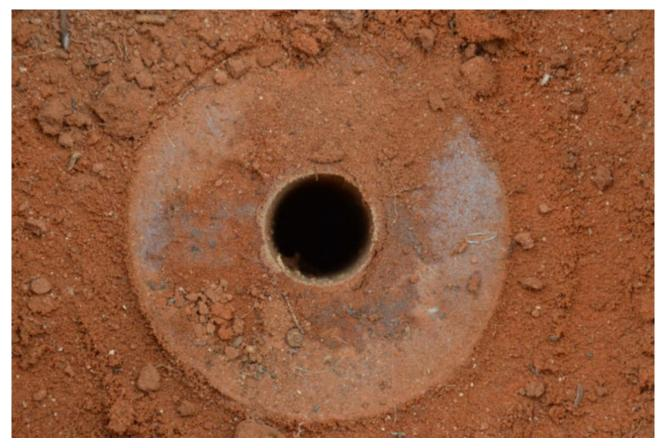
The augered hole should be circular with smooth sides visible near the top.
