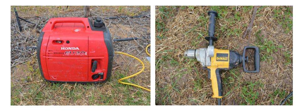
A Honda EU20 i 1.6 KVA Generator and a 740 Watt DEWALT Drill have been intensively tested to drill holes in some very heavy textured soils. These tools have not failed in the course of many installations. They are highly recommended.
