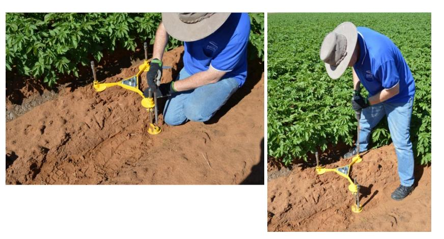
Insert screw pins into holes of tripod legs and extension foot and use electric drill to secure two tripod feet on the hill ridge and the extension foot in the furrow.
