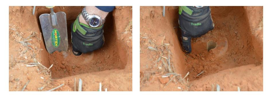
Place a finger carefully inside the augered hole to prevent soil entering and use a trowel to make a shallow 3cm deep trench to accommodate the probe cable.
