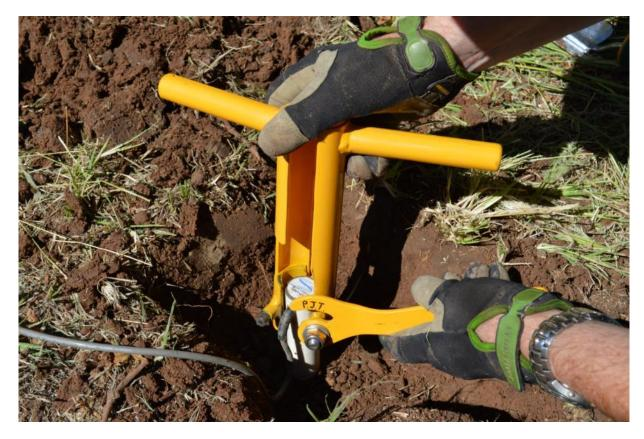
Fit the Extraction Tool around the excavated top of the probe with the probe cable located in the square opening of the extraction tool. Fold the cable down and line it up with the slit formed in the tool.
