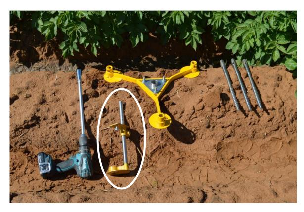
When installing the Drill & Drop probe in crops grown on hills an extension foot (circled) is used to stabilize the tripod on the hill ridge.
