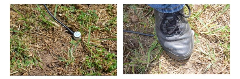
If the probe protrudes above the soil surface and you cannot push it any further by hand, gently step on it and use your body weight to push it into final position.
