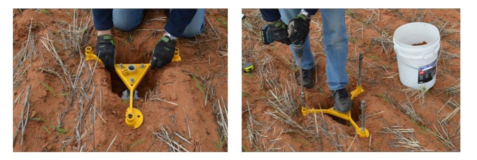
Position the Extension Tube in the centre of the excavated hole and install the Tripod Pins.
