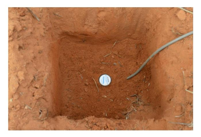
If the insertion is incomplete, then apply smooth body pressure through your foot to insert the probe to full depth. In the above example, the probe top is located 20cm below the soil surface.
