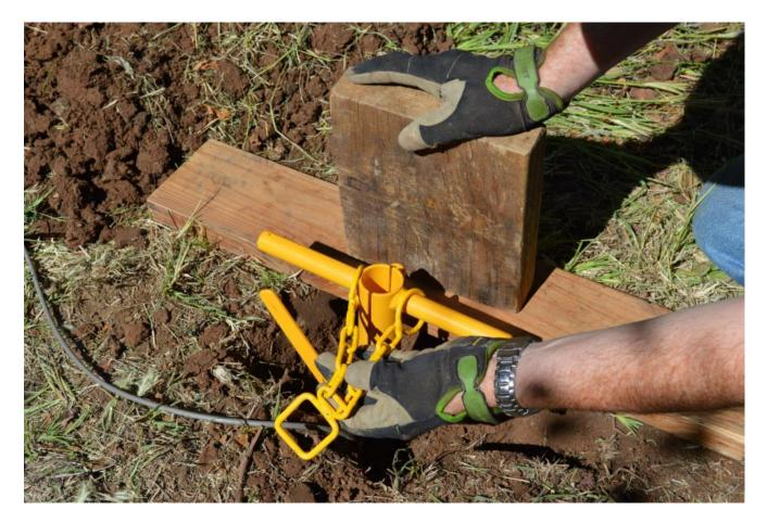
If you cannot remove the probe by hand, fit the Extraction Chain onto the Extraction Tool, one circular ring for each handle and place wooden blocks next to the probe as shown.
