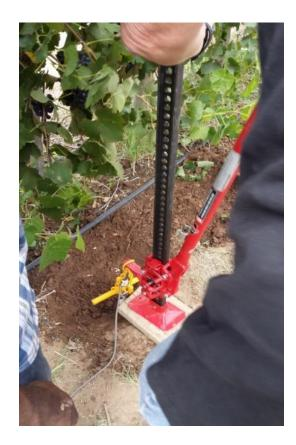
If it is not possible to remove the probe with a crowbar and blocks of wood, a High Rise Car Jack may be used.
