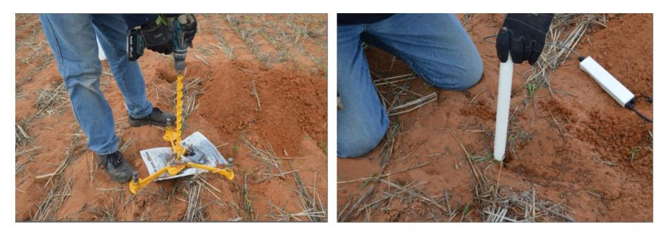
Use the 30cm Installation Auger and Tripod.
