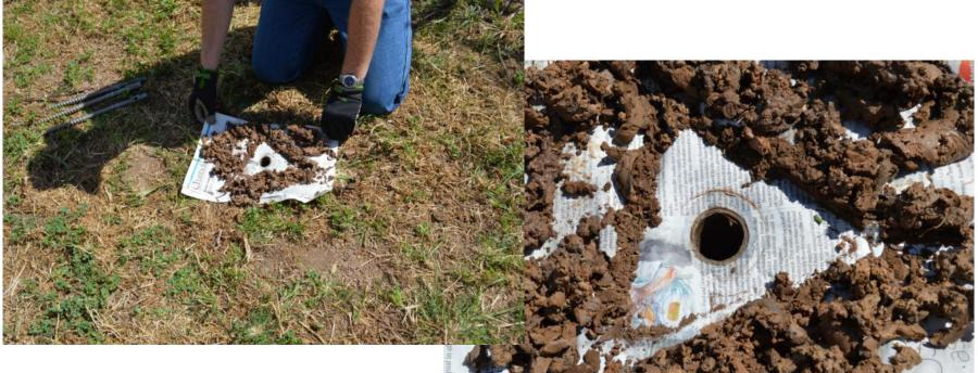
Remove the tripod and inspect the quality of the hole. It should be smooth-sided and free of air pockets.
