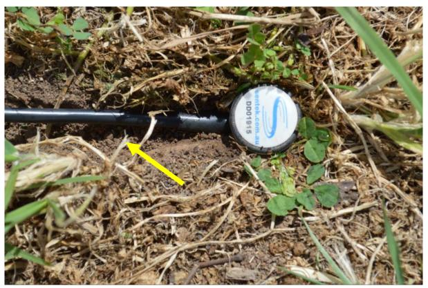
The (almost) completed installation of the probe should look like this. The probe should be in firm contact with the soil and you should not be able to push it in any further by hand.
