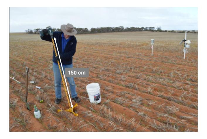
Use the <u>extended</u> 150cm subsurface auger. Measure and mark the auger at the required depth. Allow for the tripod centre height of 4cm.
