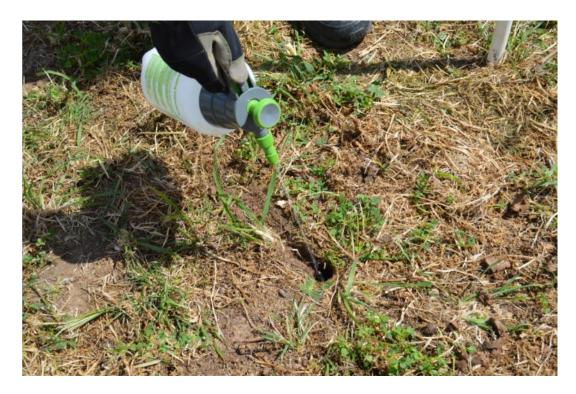
Use the spray bottle to wet the probe and the upper walls of the hole. This is particularly useful as lubrication in clay soils.
