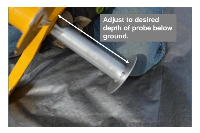
Adjust the Extension Tube to the desired depth of probe below ground and tighten the Extension Tube nut.
