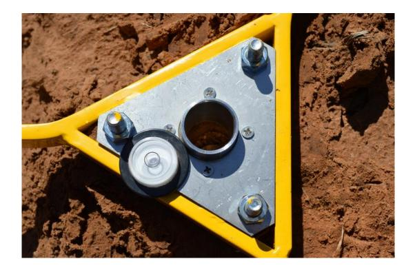
Use a levelling bubble to position the tripod correctly.
