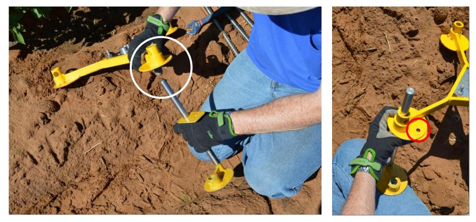
Insert the extension foot into of the tripod foot. Use the foot with the pre-drilled hole (circled).
