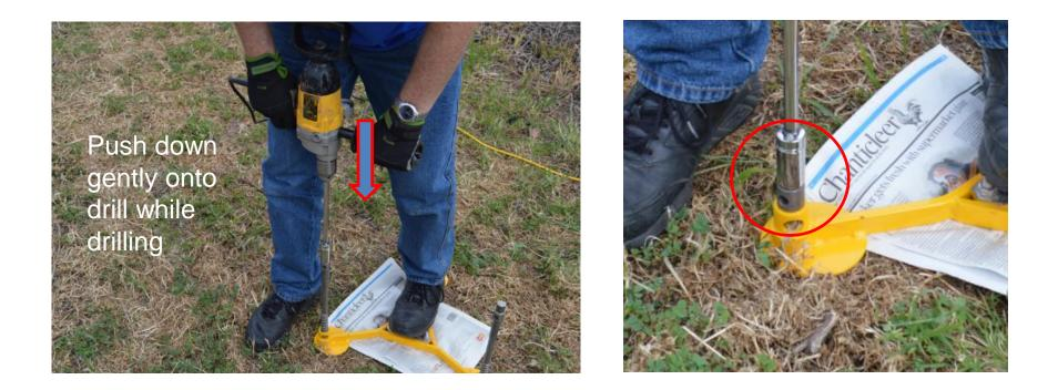
Place one foot onto the centre of the tripod, position the socket onto the screw pin and keep drilling until the head end of the pin comes to rest on top of the tripod. Repeat with the remaining 2 pins and then check the tripod stability.
