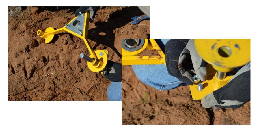
Align holes of tripod and extension foot, place bolt through the holes and tighten with the nut.
