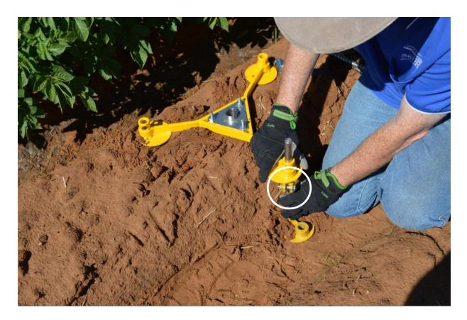
Loosen the nut and bolt of the height clamp (circled) and slide the leg to the desired height.
