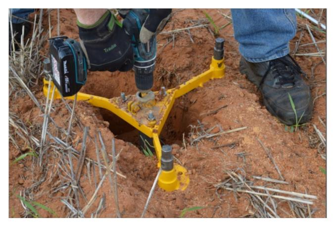
Drill to your auger mark, then carefully take the auger out, remove any soil from it and re-insert it back into the hole without rotating it. If you can insert it all the way then the hole is deep enough to receive the probe. If not then carefully auger more soil out and retest until sufficient depth is reached.
