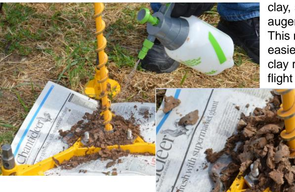
When the going gets tough in heavy clay, spray some water onto the auger and into the augered hole. This makes the drilling process easier by allowing the lubricated clay ribbons to travel up the auger flight and out of the hole.
