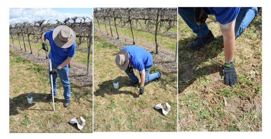
Insert the probe carefully into the hole pushing it all the way down until the top of the probe is level with the soil surface. The first sensor will now be located at 5cm depth.
