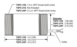
Figure 3 - Mechanical Drawing, TSPC-15S/21S/25P
