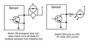
Figure 14 - Sinking Switch Output Wiring
