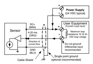
Figure 12 - Sinking Current Loop Wiring The default sourcing loop output is a 4 to 20 mA signal proportional to the measured distance between two endpoints set by the user. The current range and slope are SenixVIEW adjustable and identical to that set for the sourcing loop described above. Current flows from the power supply through the user equipment then INTO the sensor (ORG wire) as shown in Figure 12.
