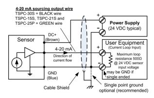
Figure 11 - Sourcing Current Loop Wiring
