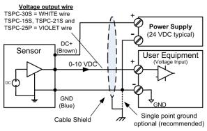
Figure 10 - Voltage Output Wiring
