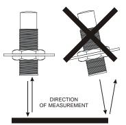
Figure 4 - Sensor Orientation
