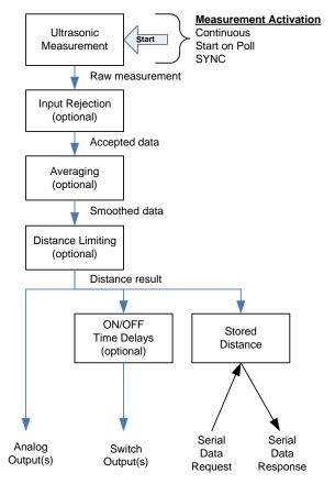
*Figure 26 - Measurement Process Diagram* In Start on Poll activation the entire process is performed once per poll, i.e., M Input Rejection x N Averaging measurements (page 35). Some filters are disallowed in Start on Poll (page 27). If a poll is received before an ongoing *measurement process* finishes, the ongoing process will run to completion then another *measurement process* will begin.
