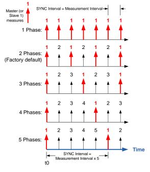
*Figure 25 - SYNC Phases and Timing* The SYNC connections use the sensor's *serial data* interface to control sensor timing and serial distance data is not available.
