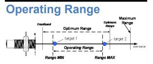
The sensor measures the distance to targets within the *Operating Range* (target 1 to target 2). This range can be set in SenixVIEW by adjusting the *Range MIN* and *Range MAX* parameters. The factory default is the widest possible, *deadband* to *maximum range* (see specifications, page 7).
