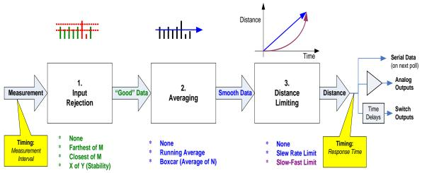
Figure 28 - Filters Block Diagram
