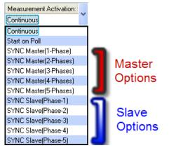
Figure 22 - Measurement Activation Selections
